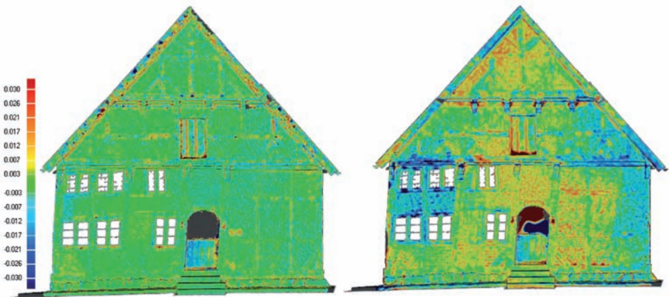
Fig. 5: Registration to the reference data of IMAGER 5006h (green < 3 mm); left: Bundler/PMVS2; right: Photofly.
