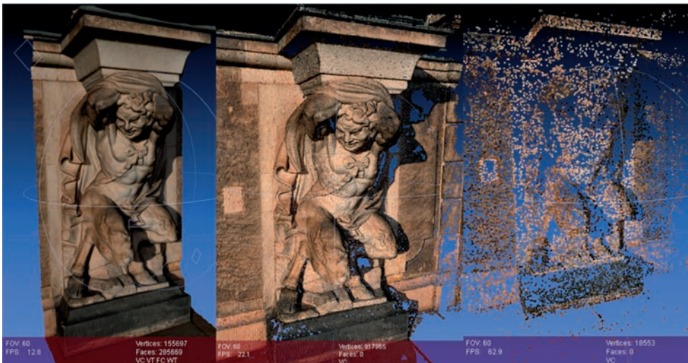
Fig. 7: Figure in the Zwinger palace of Dresden; left: Autodesk Photofly; centre: Bundler/PMVS2; right: Microsoft Photosynth.
