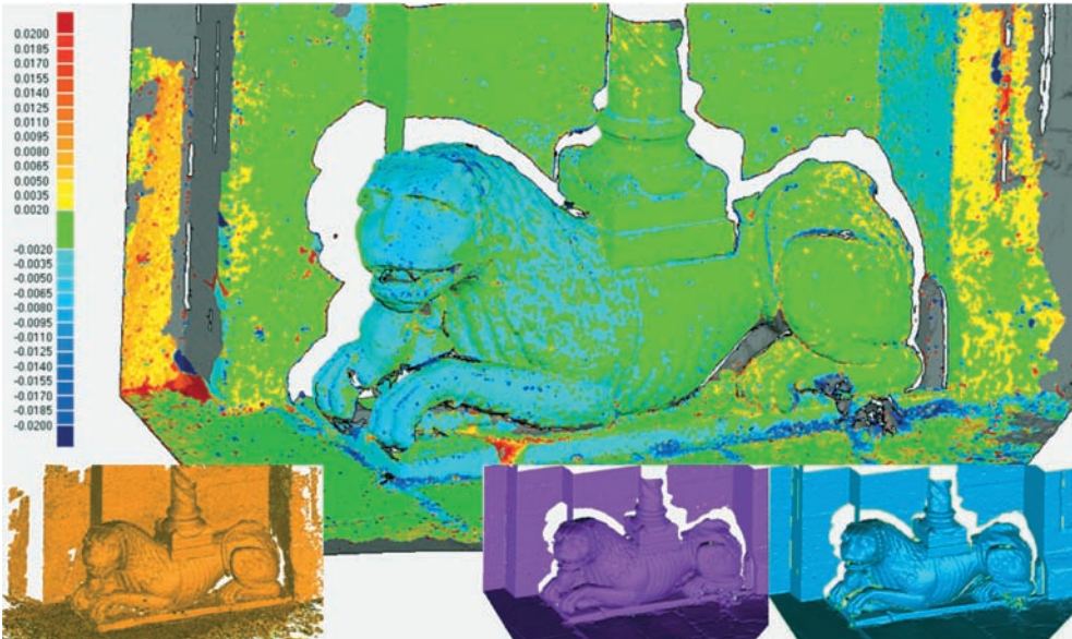
Fig. 9: 3D comparison of the lion figure at the imperial church in Königslutter between the 3D models from Bundler/PMVS2 and IMAGER 5006h; bottom left: point cloud from Bundler/PMVS2; bottom centre: IMAGER 5006h; bottom right: meshed 3D model from the IMAGER 5006h (green < 2 mm).
