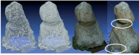
Fig. 10: Small moai (height 0.7 m) at Poike on Easter Island (Chile); left: measured points; centre left: 3D meshing; centre right: textured 3D model in each case from 123D Catch Beta; right: dense coloured point cloud measured with Bundler/PMVS2 identifying some gaps (white ellipses).
