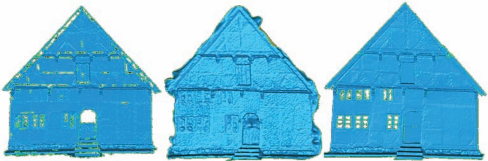
Fig. 4: 3D meshing of the front façade from the Town House in Bad Segeberg; left: Bundler/PMVS2; centre: Photofly; right: IMAGER 5006h.
