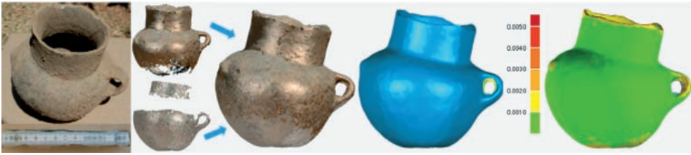
Fig. 12: Left: Photograph of the pottery from Yeha (Ethiopia) with the measuring stick for object scaling; centre left: composing the pottery from Bundler/PMVS2; centre right: meshed and smoothed 3D model of the pottery from IMAGER 5006h; right: result of 3D comparison in Geomagic Studio 12 (green < 1 mm).
