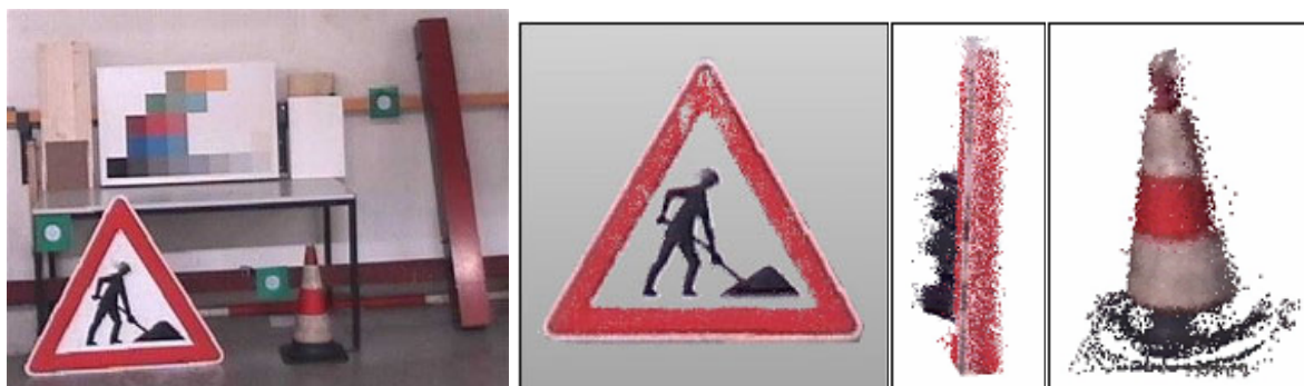
Figure 9: Different object material: overview photo (left), point cloud of a traffic sign (front and side view) (centre) and point cloud of a pylon (right)
