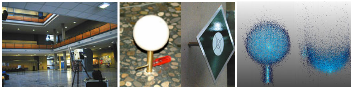
Figure 2: Mensi GS100 in the HAW 3D test field (left), sphere and target (centre) mounted on a reference point using special adapters, and scanned sphere in front and top view (right)
