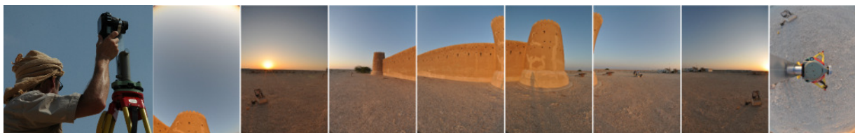
Figure 5: Camera Nikon D90 at the nodal point adapter in use (left) and eight of nine panorama images (right)
