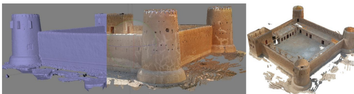
Figure 11: 3D model of the Al Zubarah fortress generated with Agisoft PhotoScan 1.0.4
