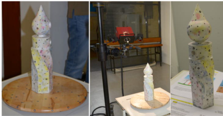
Fig. 5. Test body Testy from the Humboldt university in Berlin (left and right) and the reference scan using ATOS I 2M (centre)
