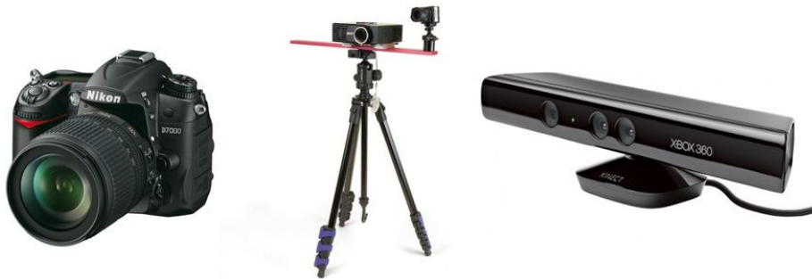
Fig. 1. Evaluated low-cost systems (f.l.t.r.): Nikon D7000, DAVID SLS-1 and MS Kinect
