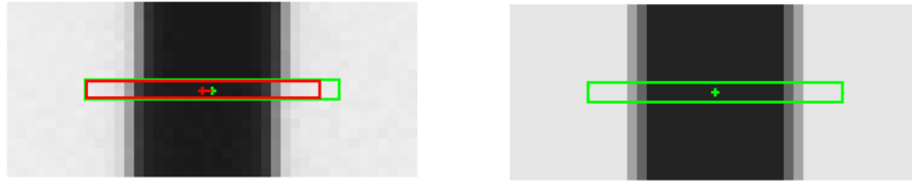
Figure 3. A broken line of the ETH plate (left). 1-D LSTM (x-shift, x-scale) with a synthetic template (right). The grey rectangle on the left is the starting value for the matching, the black one the final match position.
