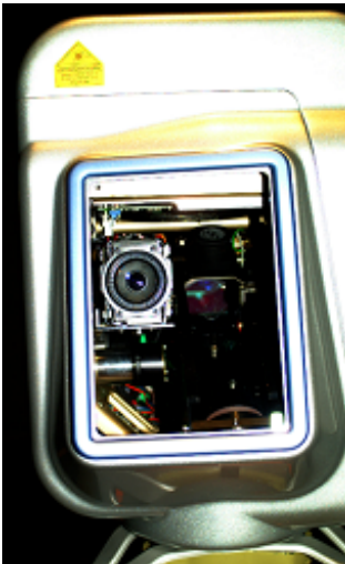
Fig. 2: View into the scanner showing the digital camera and the laser mirror
