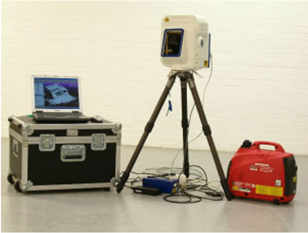
Fig. 1: The terrestrial 3D laser scanning system Mensi GS100 including transportation box, notebook and external Honda power supply at HAW Hamburg
