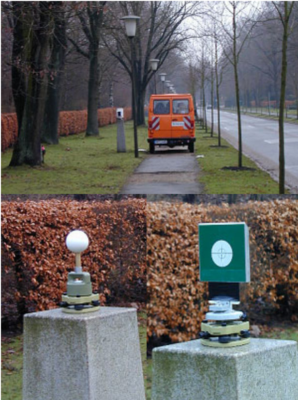
Fig. 8: Scanner on the baseline (above), sphere (left) and target (right) with the adapter used
